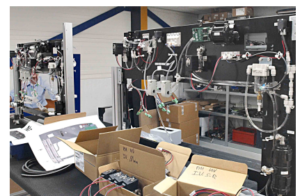
Assembling the ink management back plane.
