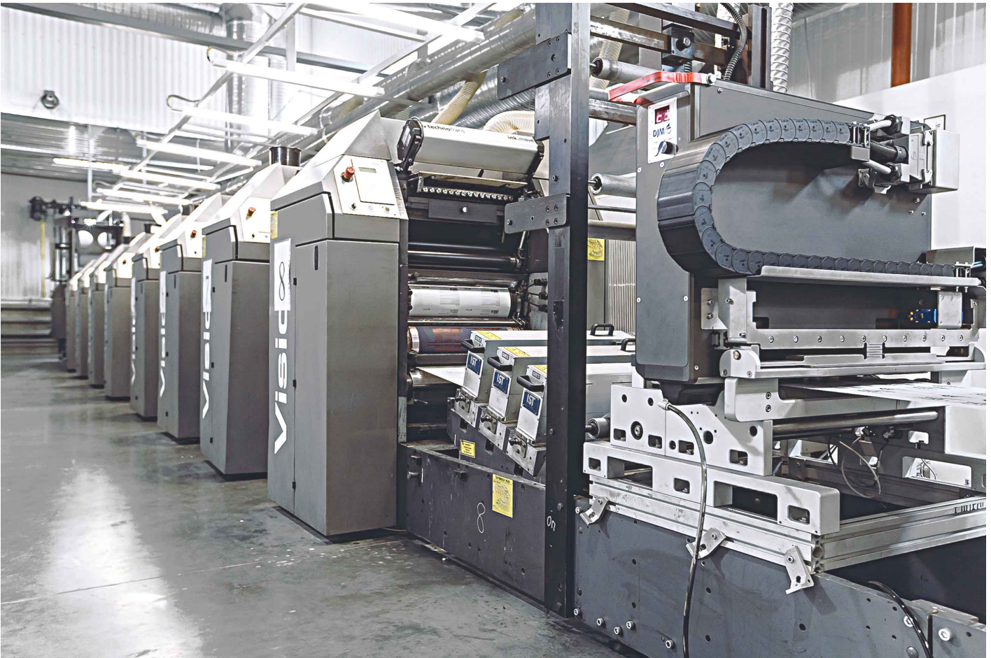
Samba print module (20,3 inches wide) integrated in web offset press.
