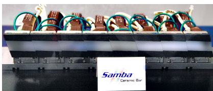
Multiple Samba printheads positioned in ceramic print bar.
