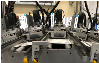
DJM's HP C800 print modules integrated on web finishing line.
